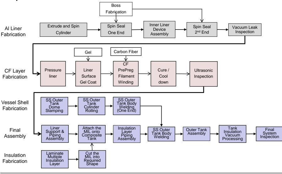
In the cryo-compressed hydrogen storage system, the top three cost drivers are the carbon fiber composite layer, cryogenic valves, and system control valves.
