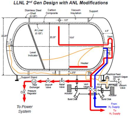
Cryo-Compressed Hydrogen Storage System Schematic<sup>1, 2</sup>
