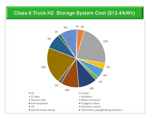
Cryo-compressed H2 tank production volume: 60,000 tanks/year (10,000 systems/year)
